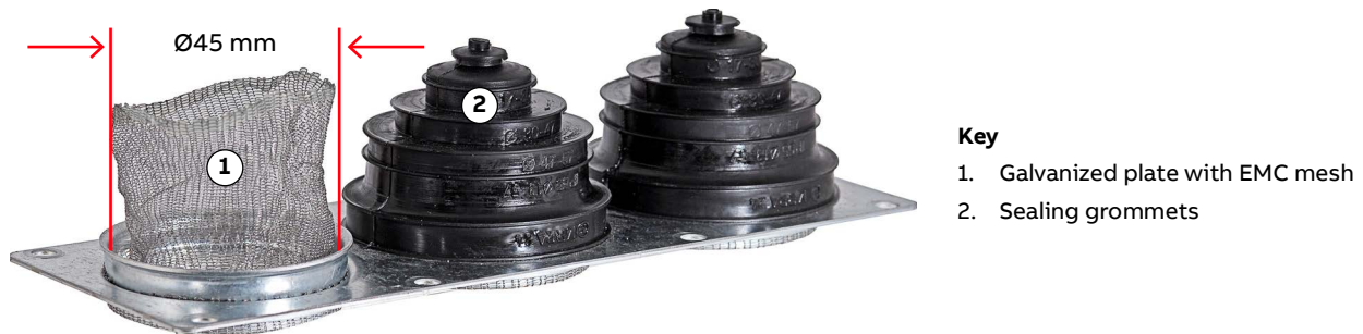
Figure 63 – Cable entry with EMC plates
